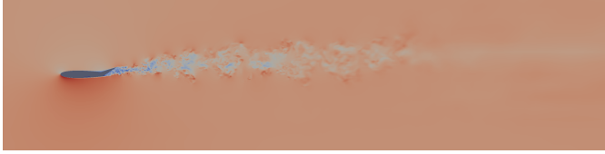
Fig. 13: Sample zoomed slice of PHASTA simulation through the wing.
